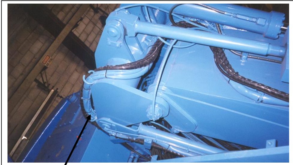
Hoses and wiring following the factory wire bundle
